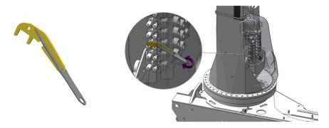
Emergency lever with the control valve V80R (stabiliser functions) You must use this side of the emergency lever to operate this control valve
