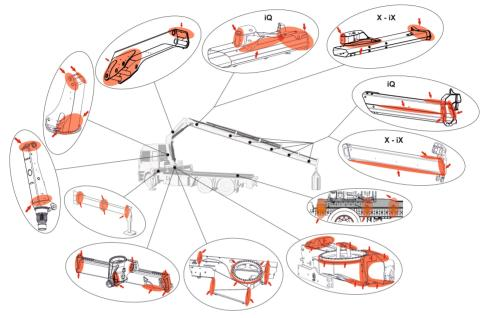
· Check for damage to the crane structure (e.g. any formation of cracks).
