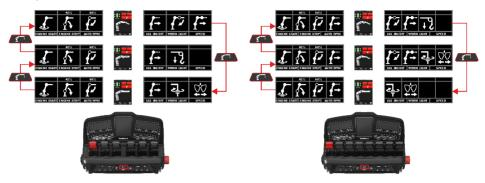
When the operator pulls out the emergency stop button on the controller, it always starts in CRANE 1 VIEW. The sub-VIEWS in CRANE VIEW are configured in production but can be changed by Effer service personnel.
