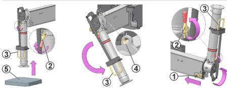
8. Retract the stabiliser extension completely. Follow the procedure: "Retract the stabiliser extensions"
