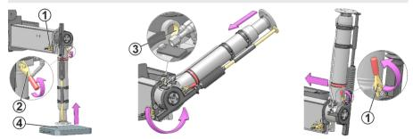
Retract the stabiliser extension completely. Follow the procedure: "Retract the stabiliser extensions"
