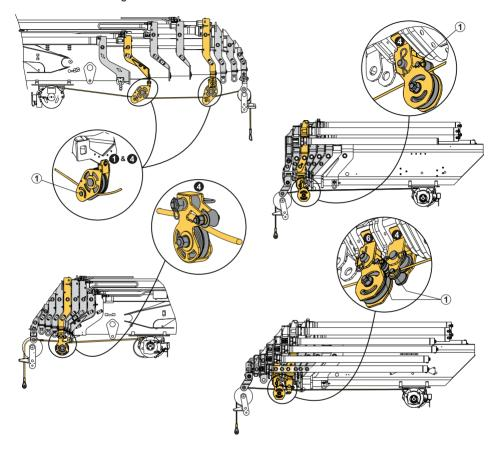
This picture shows some examples of intermediate pulleys and rope guides in different crane configuration with hoist.
