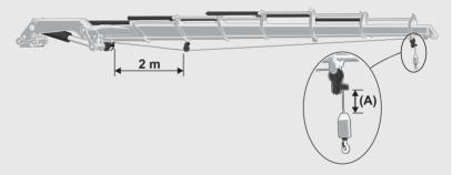
• When working with the extensions retracted, keep a minimum distance of 2m between the hoist and the rope guide on the first extension. This to avoid incorrect winding of the rope onto the drum.
