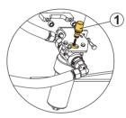
The return oil filter is on the oil tank, and can have a clogging indicator. This indicator turns red when needed. In all other cases (if the filter time is expired or without clogging indicator), you must follow the general recommendations for its replacement.
