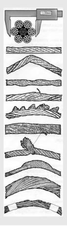
A rope has to be discarded, when there are number of ruptures in the outer layers according to DIN 15020; ISO 4309:
