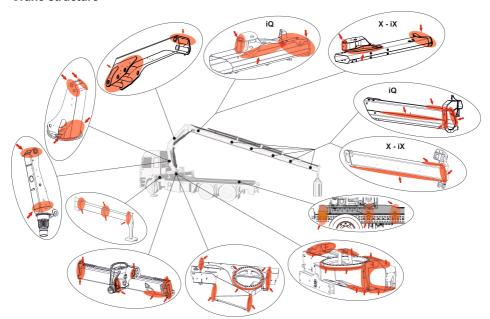
· Check for damage to the crane structure (e.g. any formation of cracks, including the paint).
