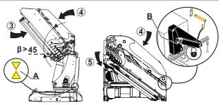
5. Lower the 1st boom completely (4) to the parking support of the base.
