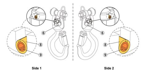
The two Spring/Roll pins (8) and (9) should be in place and nearly flush with the outer edge of the hook nut (6) on both sides. (See the pictures **Side 1** and **Side 2**).
