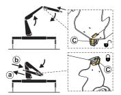
6. Lower the 1st boom completely (4) to the parking support of the base.
