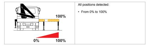
The position of the **auxiliary stabiliser extensions** is not detected proportionally by Progress to calculate the stability.
