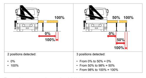
The complete crane operating area is subdivided into four sectors and their width varies according to the extension of the stabiliser extensions. Progress manages
