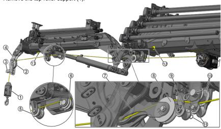
4. Remove the rope through the pulleys (5) and (6).
