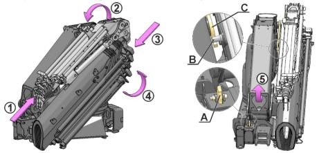
2. Raise the 1st boom (5) until BDA allows you to operate the 2nd boom or  $\beta$ >135°.
