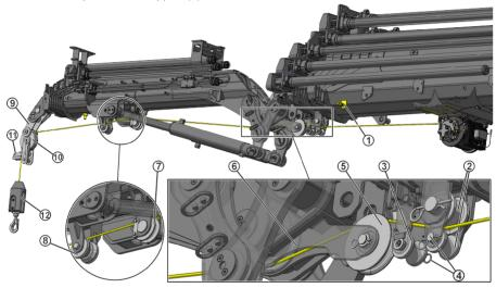
3. Put the rope through the pulleys (2) and (3):
