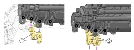
4. Attach the top-roller support for TI2L (3a) or TI4 (3b) on the last extension of the crane.
