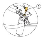
The return oil filter is on the oil tank, and can have a clogging indicator. This indicator turns red when needed. In all other cases (if the filter time is expired or without clogging indicator), you must follow the general recommendations for its replacement.
