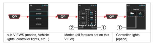
The different information shown in the alternative view depends on the crane configuration. Push the button to change between the different alternative displays for the SETTINGS VIEWS.
