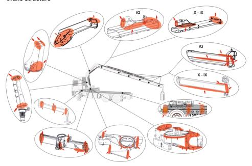
· Check for damage to the crane structure (e.g. any formation of cracks).
