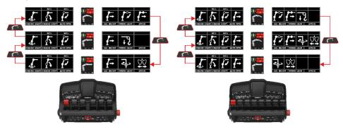
When the operator pulls out the emergency stop button on the controller, it always starts in CRANE 1 VIEW. The sub-VIEWS in CRANE VIEW are configured in production but can be changed by Effer service personnel.
