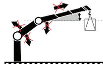
If the 2nd boom is down, the following movements are locked:
