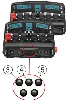
In each of the main menus the operator can step through submenus by pushing the menu button repeatedly.
