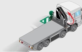
1. If the stabiliser system is manually controlled, push button
