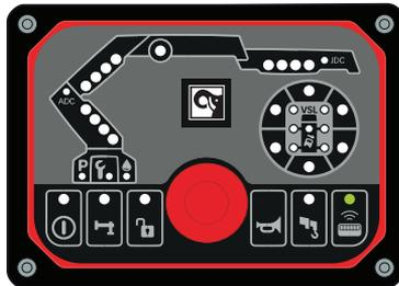
2. If using remote control, push button (1) on the controller to change the menu into crane operation.
