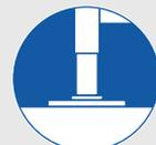
Check that the extra support plates do not bend or sink into the ground.
